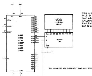
This is most useful when the outputs of the 74LS164 eight-bit shift register will be used to scan a display and/or keyboard. In this case an ANLD P7, A with A = 0FFH can be used to load the initial "1" and an ANLD P6, A with A = 0FFH can be used to move it down the shift register.
